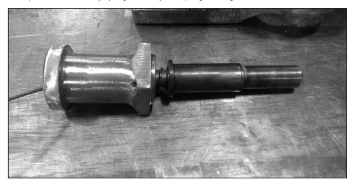
**Step 24**Apply JB Weld to end of split pin. Use emery cloth to smooth out.
