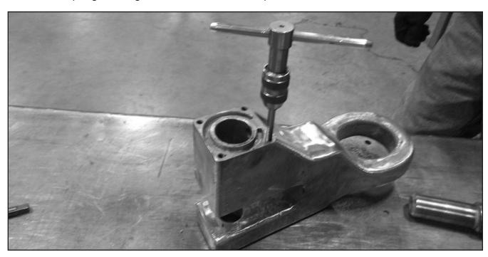
**Step 12**Clean cast housing pin holes with die grinder and carbide burr if necessary.
