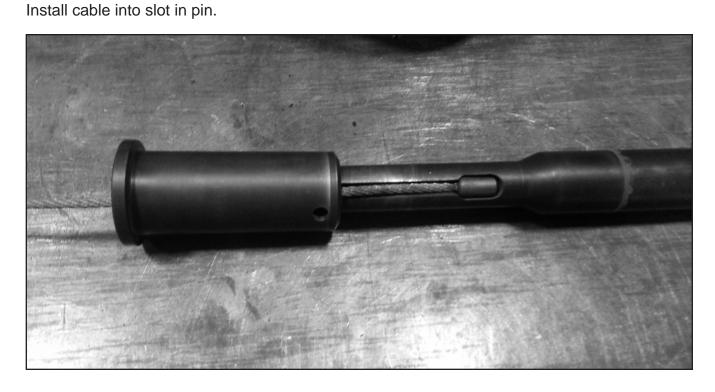
**Step 22**Align hole in sleeve with pin. Install NEW split pin.
