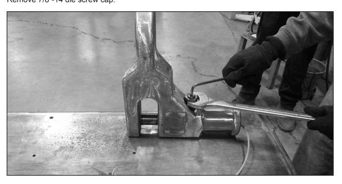
**Step 4**Remove detent housing.
