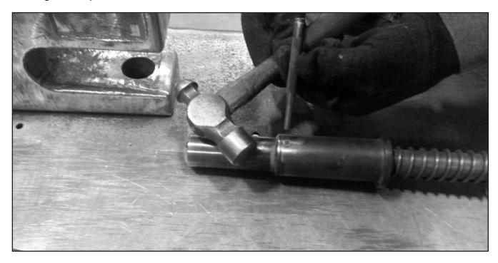
**Step 8**Set components aside. Clean and inspect for cracks or signs of fatigue or other damages.
