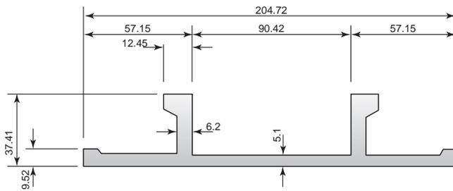
**Cross Section of Standard Vertical Rail**
