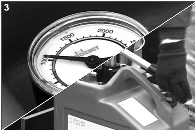
3 While holding the shore at the desired height, close the 1/4 turn release valve on pump can and pump the handle on the can to build pressure between 5.2MPa ~ 10.3 MPa.
